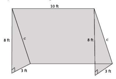
a. Determine the length of the bar, c, that would be needed to provide structure to the goal. Round your answer to the tenths place.
